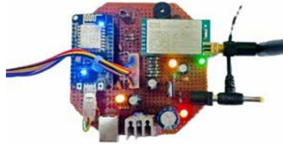
Fig. 5. SHIELD Receiver Module at Base Station
